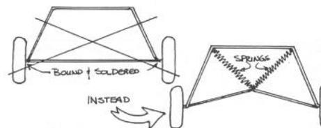
If you do want to tie the gear together, never go straight across. Instead, lash a rubber band or springs to take some of the load. The landing gear shouldn't be completely rigid, but you don't want it to jackrabbit down the field either.
