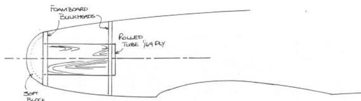
any more than that. Remember to tie the battery pack, the motor, the spar and the landing gear together. With foamboard half shell fuselages, on every bulkhead, somewhere in the middle, like with the crutch, set up a place where there is going to be a pair of lengthwise 1/8" x 3/8" pieces of spruce. This goes back and becomes the stabilizer seat and also ties into the motor tube.
