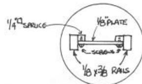
When the correct balance is achieved the plate can be secured with screws.
