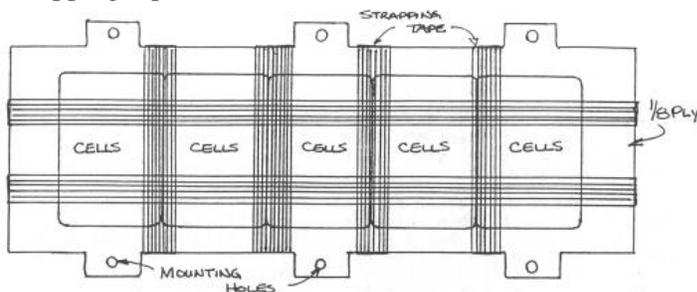
Remember those two horizontal spruce rails in the fuselage? In the battery area, I glue 1/4 inch spruce to them to allow the plate to slide in and be able to be moved back and forth. By putting a number of holes in these rails the plate can slide back and forth to change the center of gravity.
