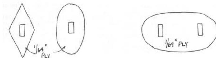
load. The load goes from the strips to the 1/64" ply and is transmitted across a larger surface of the foam board, tying them together, distributing the load.
