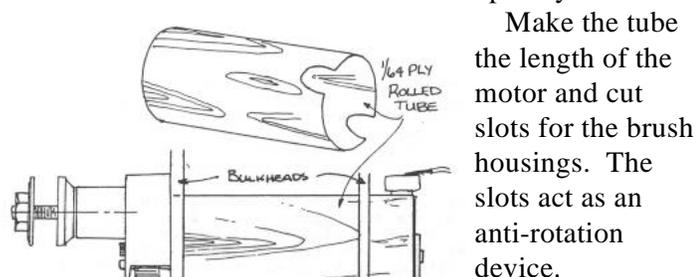
Make the tube the length of the motor and cut slots for the brush housings. The slots act as an anti-rotation device. Another trick is to trap the motor with the gearbox. The motor can't move back and forth. Without the gear box, a snug fit is achieved by putting a strip of masking tape on the motor and pushing it into the motor mount for a snug friction fit.
