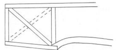
If you think about it, as you come into land, the motor wants to continue down and this diagonal, in compression, prevents the bay from parallelogramming. The triangle is doing its job. You can also put one going the other way.
