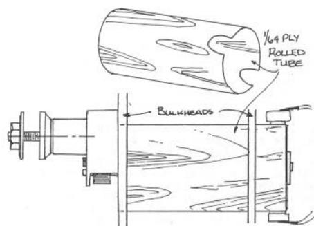
Another trick is to trap the motor with the gearbox. The motor can't move back and forth. Without the gear box, a snug fit is achieved by putting a strip of masking tape on the motor and pushing it into the motor mount for a snug friction fit.
